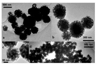
Figure 2. Foamlike balls composed of platinum nanosheets and their aggregates
