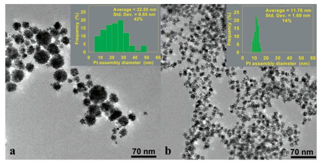
*Figure 4.* TEM images of platinum nanostructures produced in the presence of SDS without (a) and with (b) photocatalyst and their respective size distributions (insets). Average diameters were measured for 100 nanostructures, and their frequencies are plotted in the inset graphs. The average size and the standard deviations are given in the plots, along with the percentage ratio of the standard deviation to average size.
