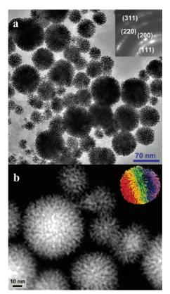
Figure 3. (a) TEM image of nanodendrites produced with Brij-35 surfactant in the absence of photocatalyst and (inset) the electron diffraction pattern of a group of the dendrites indicating that they are composed of platinum metal and as a group are polycrystalline. (b) HAADF scanning TEM image of the three-dimensional platinum dendrites grown in the presence of Brij-35 micelles. Inset: a Koosh ball.
