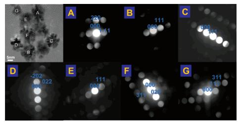
*Figure 9.* High-resolution TEM image showing several labeled nanodendrites and their convergent beam electron diffraction patterns. The electron diffraction patterns verify that the nanostructures are single crystals and that each nanodendrite has a different orientation on the TEM grid. The indexing gives the different crystallographic orientations of the individual nanostructures.
